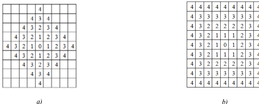
Fig. 2. Distance map from the center pixel: a — d_4 distance; b — d_8 distance
