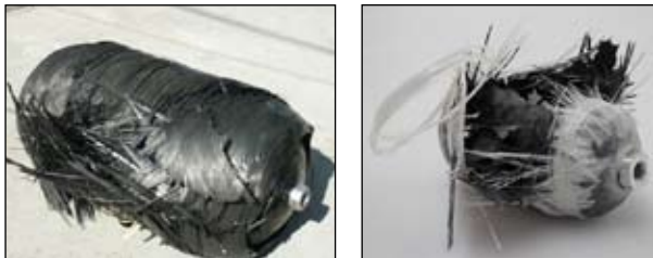
Fig. 6. Results of kevlar composite tank explosion
